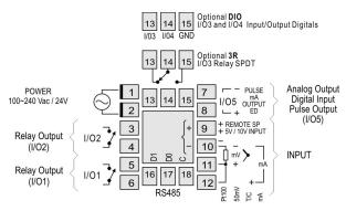
Figure 1 - Connections of the back panel
